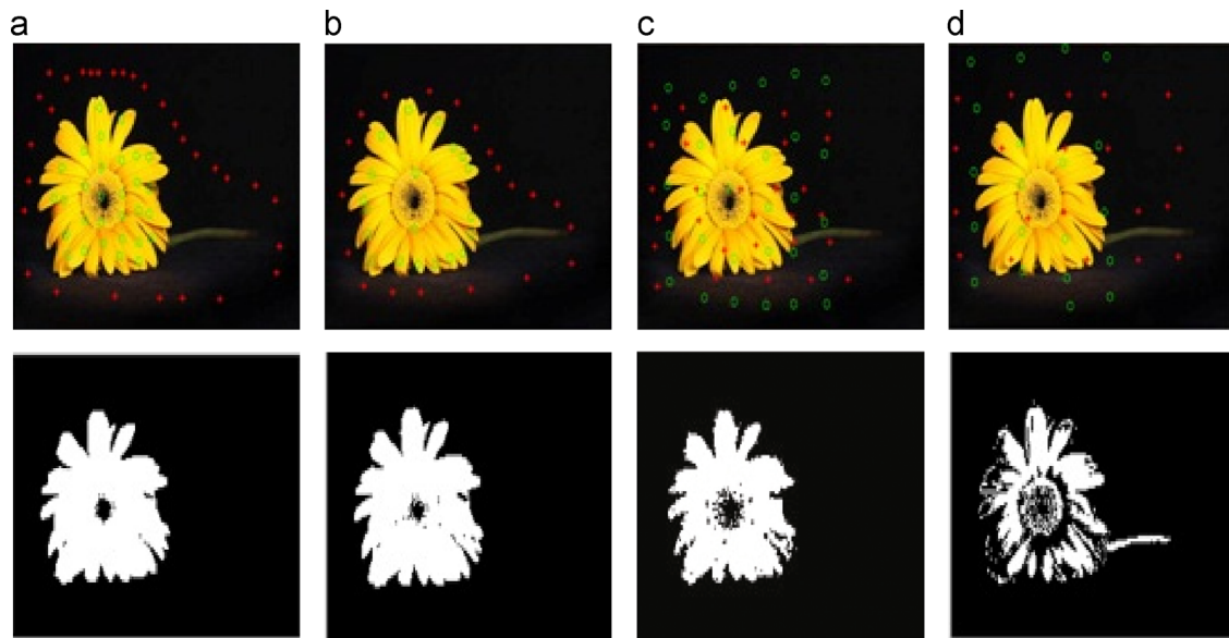
Fig. 6. Segmentation results comparison of different number training pixels by ISVM method. (a) 60 right specified training pixels; (b) 40 right specified training pixels; (c) 60 wrong specified training pixels; (d) 40 wrong specified training pixels.
